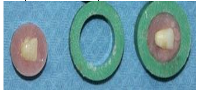
Fig. (1): Crowns were embedded horizontally in middle of the mould.
