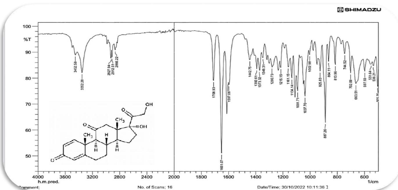
**Figure (3):** FTIR spectrum for pure PRD powder
