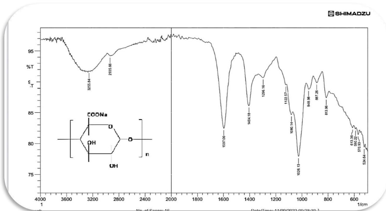
Figure (4): FTIR spectrum for pure S. Alg powder.
