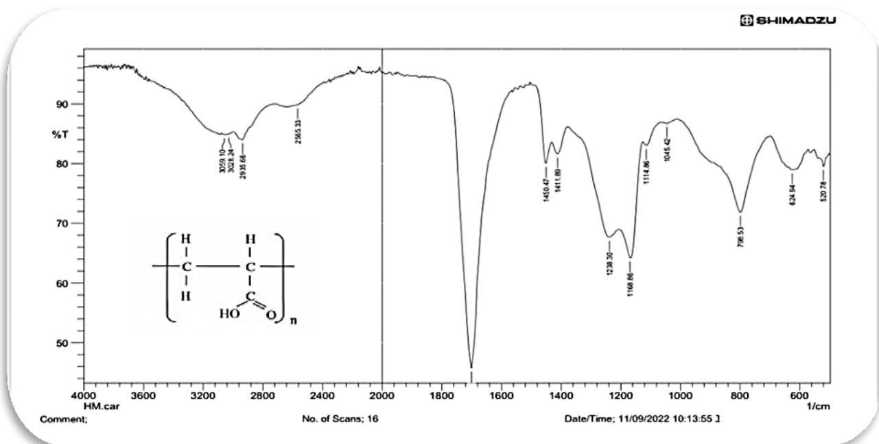
Figure (5) FTIR spectrum for pure carbopol 940 powder
