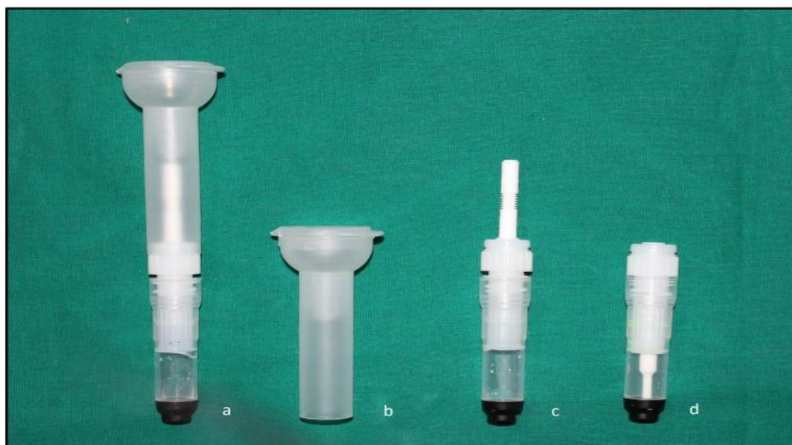
Figure 2: HY-Lite 2 Surface Testing Pens. (a) An unused surface testing pen on the left and a used pen on the right. (b)- Protection cap with integrated rinse solution, (c)- White sampling stick, (d)- Cuvette filled with test buffer and Reagent chamber sealed with aluminium foil, containing freeze-dried and stabilized luciferin/luciferase mixture.
