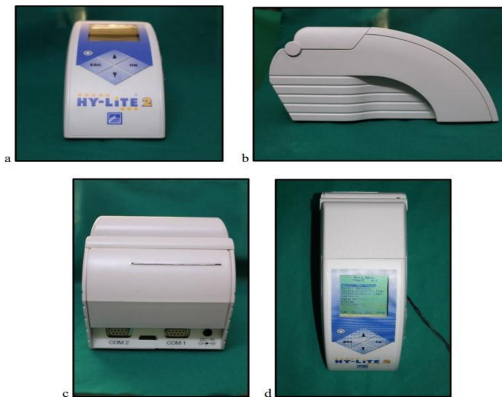
Figure 1: HY-Lite 2 ATP Bio luminometer (Merck, Germany) (a) Frontal view, (b) Lateral view, (c) Back view showing attachment points. (d) Aerial view
