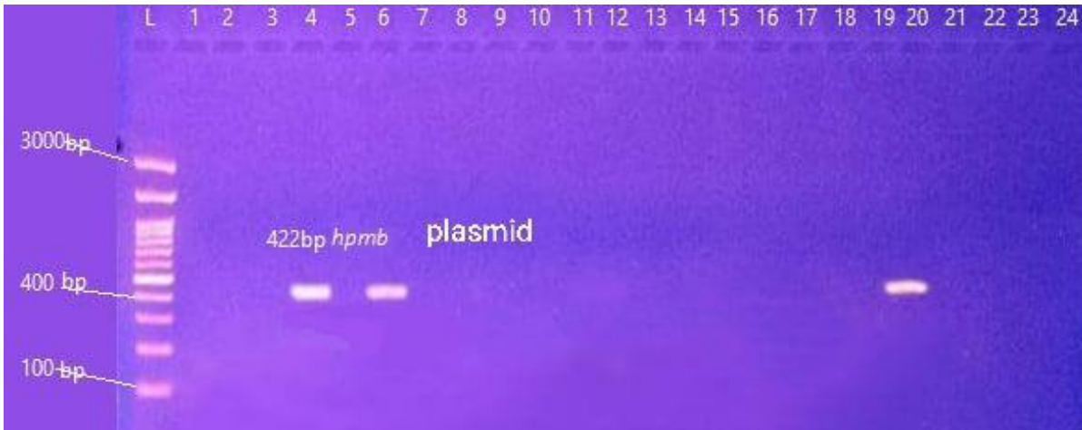
Figure 4: Agarose gel electrophoresis of amplified hpmB gene PCR product (422 bp) in plasmid (L: DNA Ladder 100-3000 bp, Agarose: 2%, Volt: 100v, Lanes showing (4, 6, and 20) represent bands of P. mirabilis isolates.
